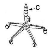
2. Insert gas cylinder into center of base.
