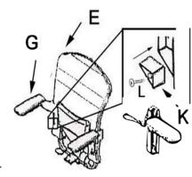
Slide armrests onto notched sides of backrest & screw in both K - Armrest Stoppers using one L screw each.
