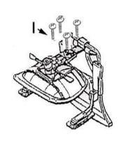
5. ) Connect backrest to mechanism using four I bolts.
