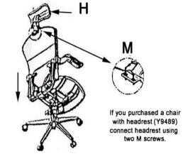
6.) Connect the seat/back upper portion and base/gas cylinder lower portion together by lining up with hole in mechanism. Set upper portion over lower portion and push down. Carefully sit in the chair to pressure fit together.
