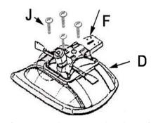
3.) Attach mechanism to seat cushion using four J bolts.
