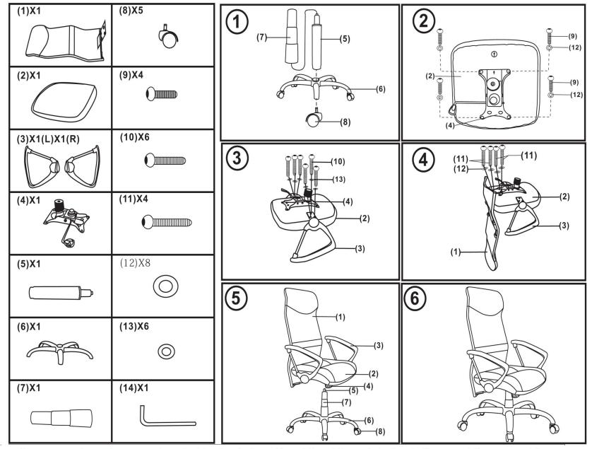
Screws and washers are located in the holes. Use Allen Wrench to back them out for assembly.
