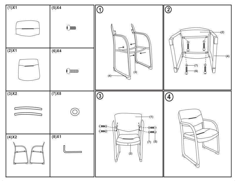
Screws and washers are located in the holes. Use Allen Wrench to back them out for assembly.
